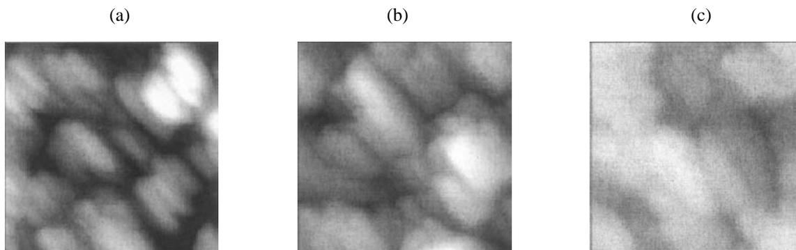
**Fig. 2.** Carbon-modified LDPE surface; the frequency of pulse generation by the carbon plasma generator 1 Hz. Number of pulses  $N$ : (a) 10, (b) 50, and (c) 100. Coating thickness, nm: (a) 1.5, (b) 7.5, and (c) 15.0.
