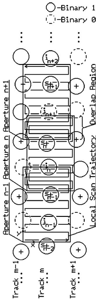
FIG. 1. PSD bit track. Information elements  $i_n$  are separated by synchronization elements  $s_n$ . The “+” sign marks the positions of synchroelements relative to which the rectangular aperture local positioning is carried out.
