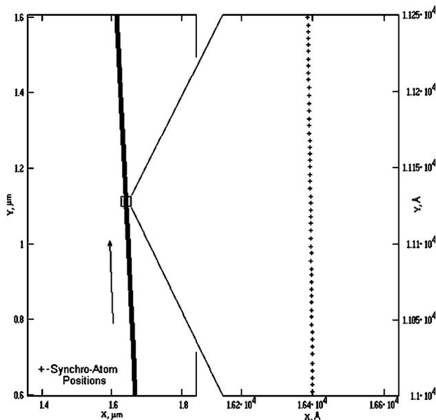
FIG. 2. Displacement of the STM probe along a crystallographic direction by a chain of 2048 carbon atoms serving as the bit track synchroelements. The atoms located between synchroatoms are informational (not shown), in this case they are all binary 1's. The path length distance is  $\approx 1 \mu\text{m}$ . The readback rate is 33 infoatoms/s. The number of probe attachment failures is 0. The arrow points to the direction of probe movement.
