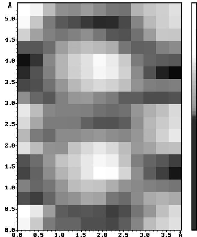
FIG. 3. A  $13 \times 18$  aperture. The image is smoothed. The carbon atom at the top of the aperture acts as a synchroelement and the atom at the bottom acts as an infoelement. Constant  $Z$  mode,  $U_{\text{tun}}=50 \text{ mV}$ ,  $I_{\text{tun}}=993 \text{ pA}$ . The number of samples per point is 1. The scan velocity is  $294 \text{ nm/s}$ .
